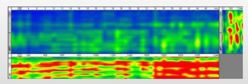
Thinning of the plate: wall thickness decrease from 100 mm to 50 mm is observed
