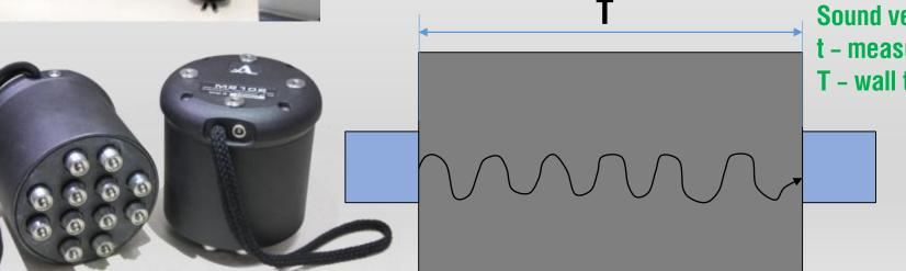
Sound velocity V = T / t t - measured propagation time T - wall thickness
