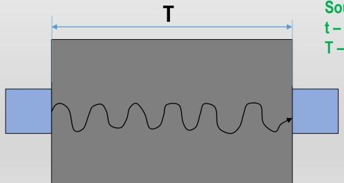
Sound velocity V = T / t t - measured propagation time T - wall thickness
