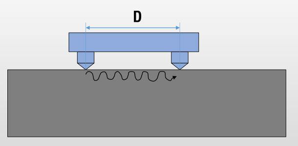
Sound velocity V = D / t t - measured propagation time
