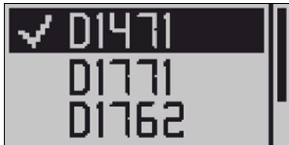
The currently calibrated probe is indicated by a marker . Use and to navigate through the list of available probes.
