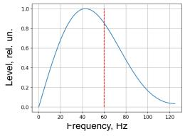
Operating frequency  $f_c$ : 43.4 kHz AFC maximum  $S_{rel}$ : -50.9 dB Absolute transmission bandwidth P: 62.6 kHz Relative transmission bandwidth  $B_w$ : 117 %
