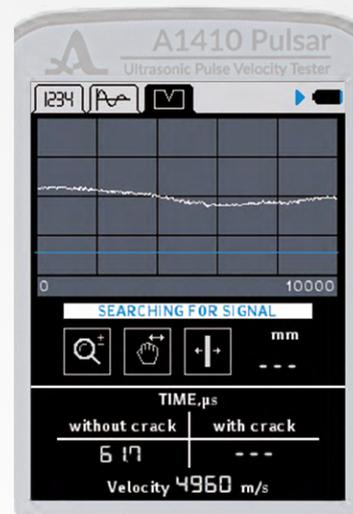
Figure 42: Device ready for crack measurements
