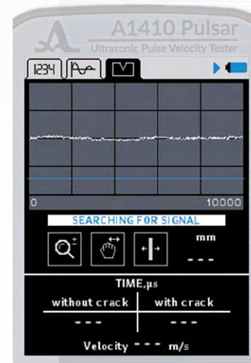
Figure 38: Crack Sizing Mode screen before calibration
