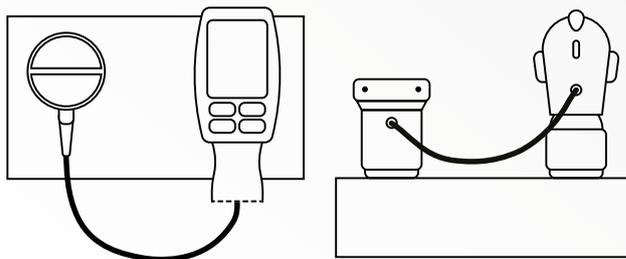
**Figure 3: Correct arrangement of transmitter and receiver unit**
