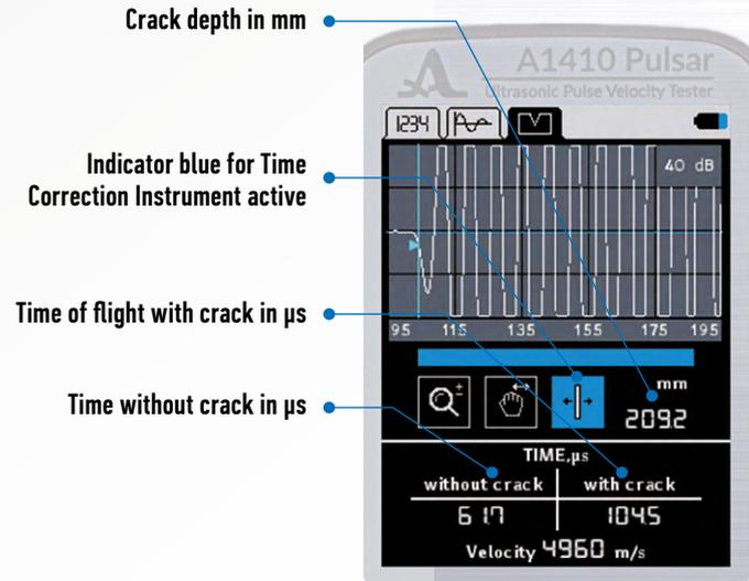
Figure 44: Displayed data after measurement
