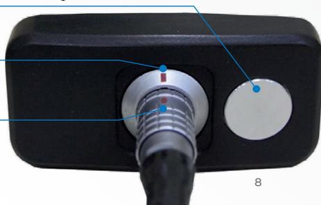
On the lower end surface of the electronic unit there is a lug for the belt, USB Micro B connector used for the USB connection of the communication cable to a PC, and a connector for connection/disconnection of the power adapter to charge the built-in battery (Figure 3).
